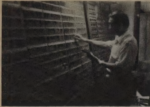
A print shop in Taipei, Taiwan, 1987. The typesetter is selecting type from an entire wall of characters.
